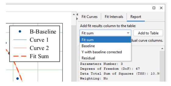
Column(s) from the selected curve(s) (including Fit Sum) can be added to the Table using the context menu of the Curve itself in the plot area or in the curves list or from the context menu of the legend symbol:
