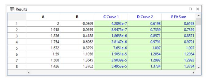
The created columns have links to the Fit Plot. The Auto Recalculation is on by default for the created columns and can be switched off.
