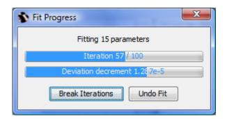
MagicPlot shows current iteration number and deviation decrement with two progress bars while fit is performed. The fit process stops when one of these progress bars reaches the end.
